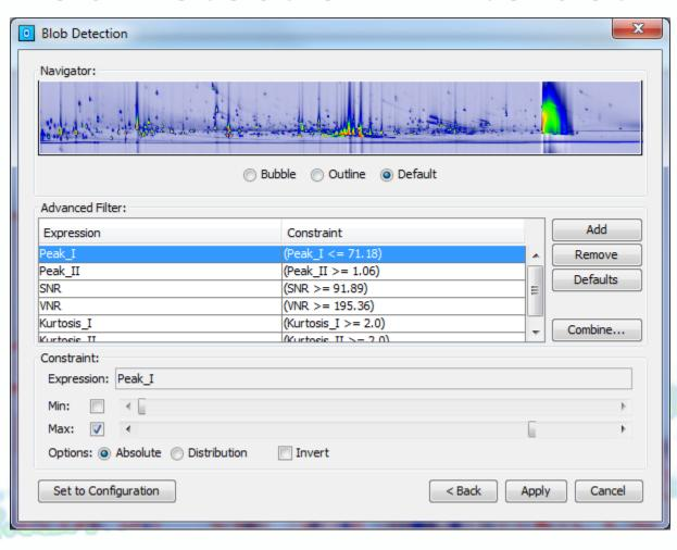
Filters are applied in combination. As a filter is changed, e.g., with slider, blobs are added or removed.
