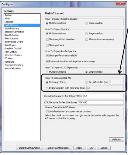
User-controlled configuration. Integration within dynamic bins uses large intensity ions as a tentpole around which smaller intensities within the tolerance are integrated.
