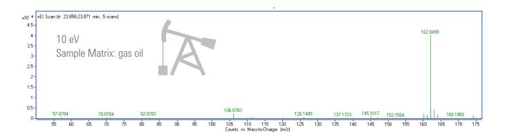
Spectral ambiguity is reduced with revolutionary Low Energy El on the 7250 GC/Q-TOF. Based on the High Efficiency Source found on 5977 HES GC/MSD and 7010 GC/TQ platforms, the Low Energy capable El source greatly maintains compound sensitivity while enabling a spectral tilt towards molecular ion. This example shows 3,5-dimethylbenzothiophene detected in gas oil, with identification facilitated by use of Low Energy El.
