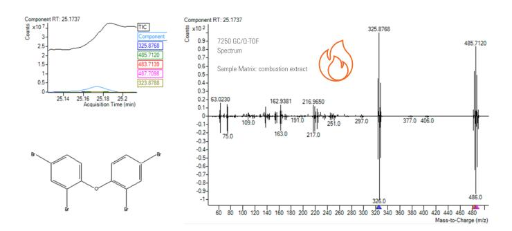
MassHunter Unknowns Analysis software, using SureMass signal processing, provides insight and accuracy beyond conventional deconvolution techniques. Even minor components are accurately extracted and identified in the presence of dominating background signal. The data shown here depicts the trace detection of dibromophenyl ether with a match score of greater than 95 in complex combustion byproducts.
