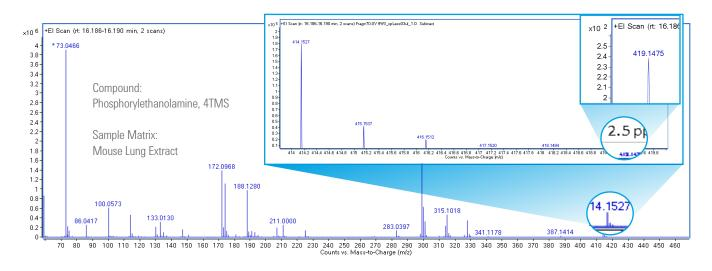
A wide in-spectrum dynamic range enables confident detection of trace level analytes in the presence of abundant background or other coeluents.
