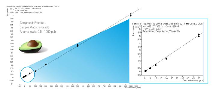
A wide linear dynamic range brings quantitative accuracy across a range of compound concentrations. Response factors are maintained even at low concentrations in a complex sample, as shown in this data depicting Fonofos at 0.5-1000 ng/mL in an avocado matrix.
