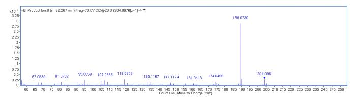
With MS/MS product ion spectra generated from a putative molecular ion, powerful Molecular Structure Correlator software can propose compound structure possibilities and likelihoods based on fragment data.
