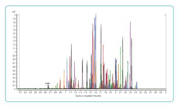
**Q-TOF identification of 100 pesticides in less than three minutes.** Superior peak capacity and fast MS acquisition lets you resolve large numbers of pesticides and ensures high confidence in compound identification. The fast acquisition capability of the Q-TOF allows considerably shorter run times while still acquiring full spectral data. (1290 Infinity LC using a ZORBAX RRHD column and 6540 Accurate-Mass Q-TOF)
