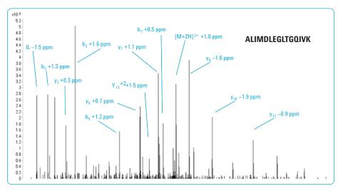
An MS/MS spectrum is shown for a peptide, ALIMDLEGLTGQIVK, from <u>Schizosaccharomyces pombe</u>. All b- and y- ions from the peptide are shown with corresponding mass accuracy values. (Agilent HPLC-Chip/MS and 6538 Accurate-Mass Q-TOF)
