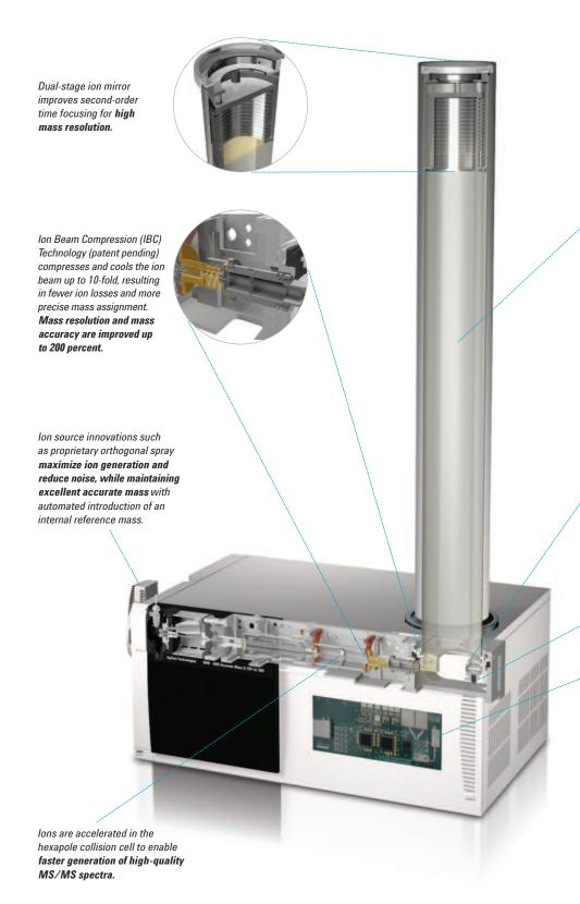
Proprietary INVAR flight tube sealed in a vacuum-insulated shell eliminates thermal mass drift due to temperature changes to maintain excellent mass accuracy. Added length improves mass resolution.
