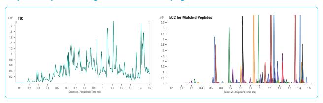
Complete mAb sequence coverage in less than two minutes. This example shows extracted compound chromatograms (ECC) for peptides matched to the lgG sequence; for both light and heavy chains, 100 percent sequence coverage was obtained. At a flow rate of 1.6 mL/min with system pressure of >1100 bar, analysis time was under two minutes. (Agilent 1290 Infinity LC using a Poroshell 120 column and 6530 Accurate-Mass Q-TOF)
