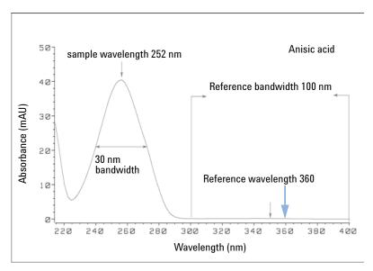
Figure 19 Optimization of Wavelength Setting
