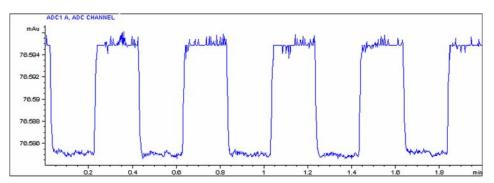
Figure 46 D/A Converter (DAC) Test – Example of Integrator Plot
