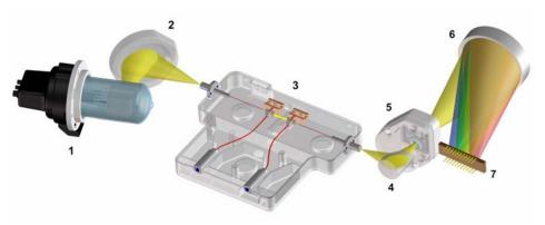
Figure 3 Optical System of the Detector
