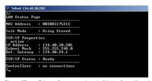
Figure 67 Telnet - Current settings in "Using Stored" mode
