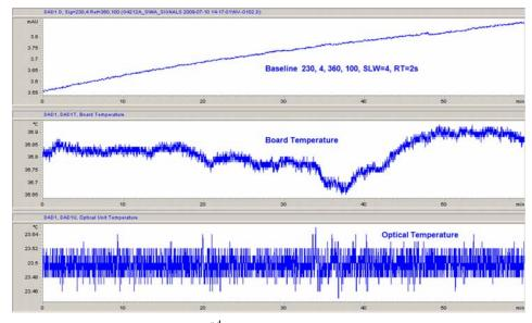
**Figure 30** Detector Warm-up – 2<sup>nd</sup> hour
