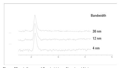
Figure 20 Influence of Bandwidth on Signal and Noise
