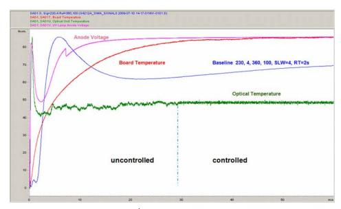
Figure 29 Detector Warm-up – 1<sup>st</sup> hour
