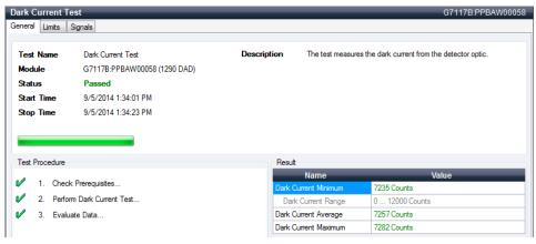
Figure 47 Dark Current Test – Results
