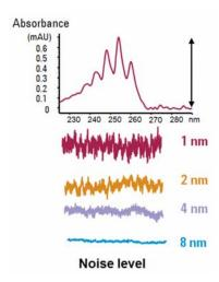
Figure 7 Influence of slitwidth on resolution and noise level
