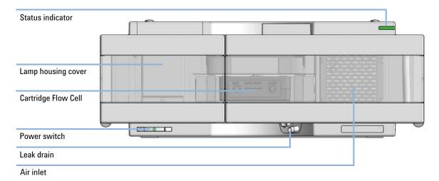
Figure 2 Overview of the Diode Array Detector
