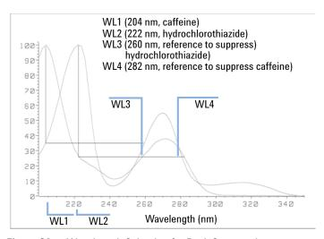
Figure 24 Wavelength Selection for Peak Suppression
