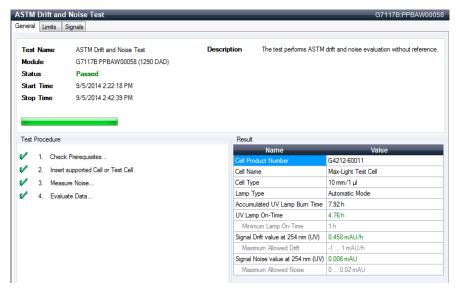
Figure 39 ASTM Drift and Noise Test – Results
