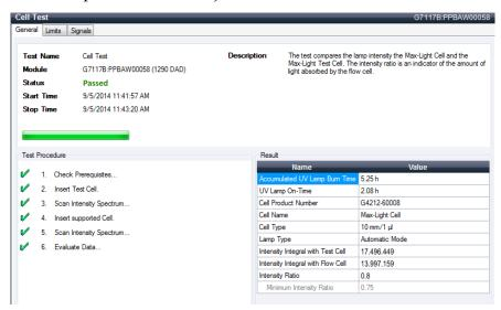
Figure 35 Cell Test – Results
