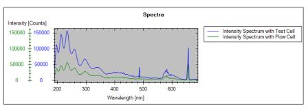
Figure 36 Cell Test – Signals (example shows low intensity for flow cell)
