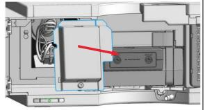
4 Unplug the lamp connector (1.) and unscrew the two lamp screws (2.) (Pozidriv).
