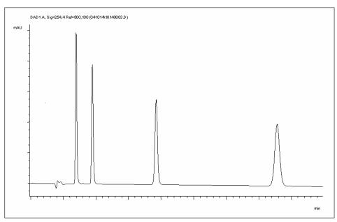
Figure 17 Chromatogram with Isocratic Test Sample
