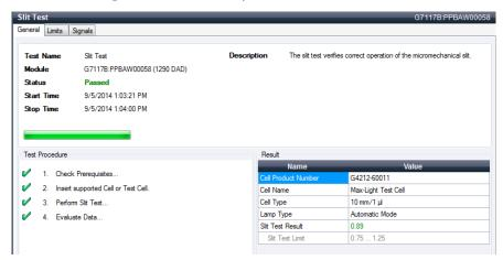
Figure 41 Slit Test – Results
