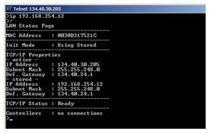
Figure 68 Telnet - Change IP settings
