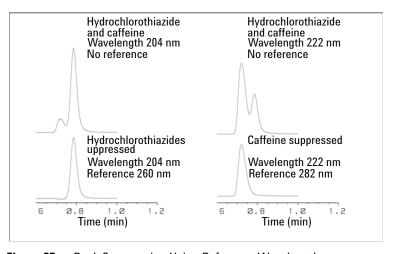
Figure 25 Peak Suppression Using Reference Wavelength
