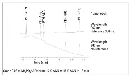
Figure 21 Gradient Analysis of PTH-Amino Acids (1 pmol each), with and without Reference
