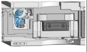
**9** Slide the lamp cover into the top position of the metal front (1.) and press the lamp cover completely in until it clicks (2.).
