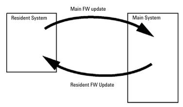
Figure 50 Firmware Update Mechanism
