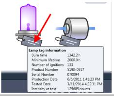
RFID tag information is displayed when moving with the mouse cursor on to the tag attached to the flow cell or lamp. The information provides flow cell and lamp related information like
