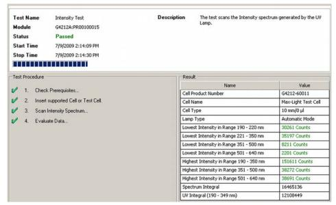
Figure 33 Intensity Test – Results
