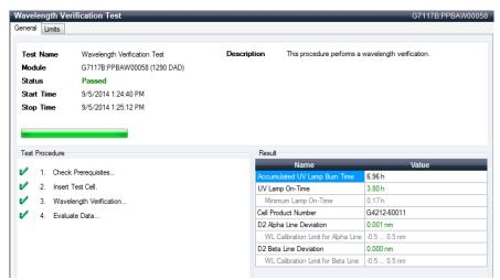
Figure 43 Wavelength Verification – Results
