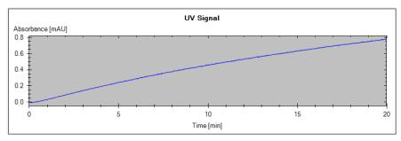
Figure 40 ASTM Drift and Noise Test – Signal
