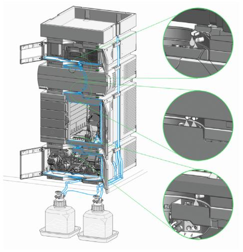
Figure 9 Leak and waste handling concept (overview - typical stack configuration as an example)
