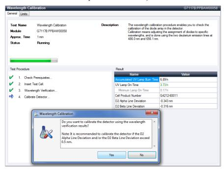
Figure 44 Wavelength Calibration - Results
