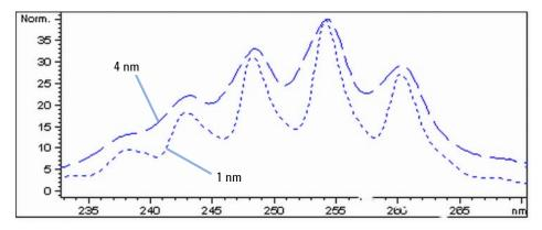
Figure 22 Benzene at 1 and 4 nm slit width (principle)
