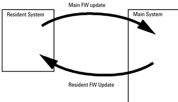
**Figure 50** Firmware Update Mechanism
