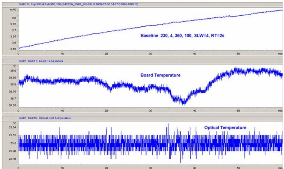
Figure 30 Detector Warm-up – 2<sup>nd</sup> hour
