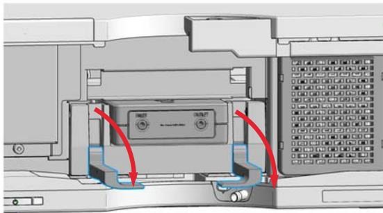
4 Pull the cartridge holder completely out.
