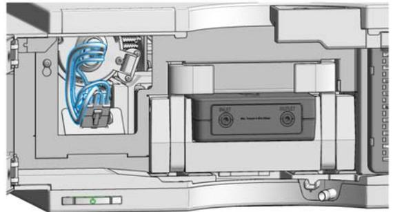
**9** Slide the lamp cover into the top position of the metal front (1.) and press the lamp cover completely in until it clicks (2.).
