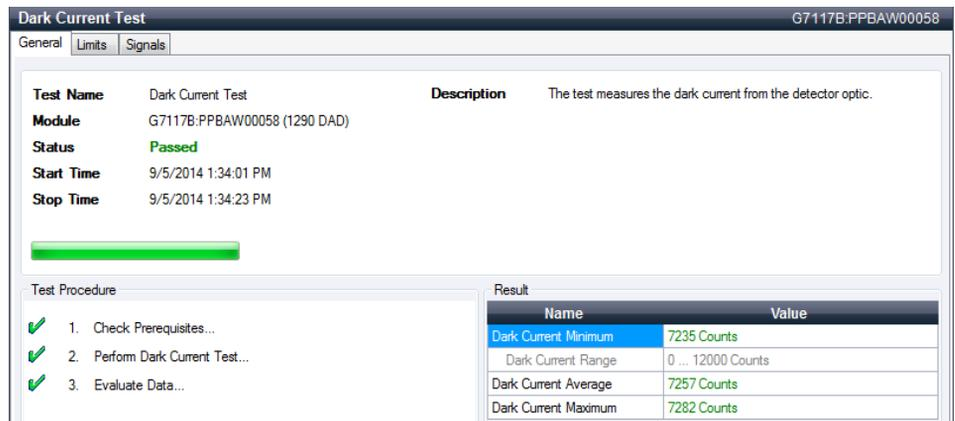
**Figure 47** Dark Current Test – Results
