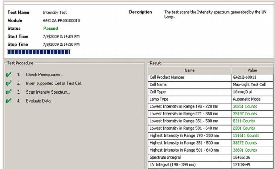
Figure 33 Intensity Test – Results
