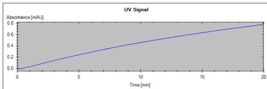
**Figure 40** ASTM Drift and Noise Test – Signal
