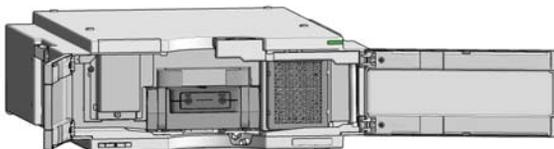
**2** Use tissue to dry the leak sensor area (1). Observe the capillary connections and the flow cell area (2) for leaks and correct, if required.
