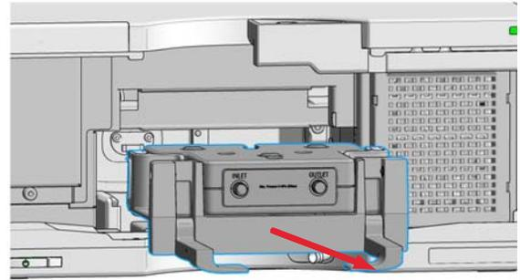
5 Remove the flow cell cartridge.
