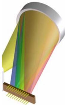
**Figure 8** Grating and diode array
