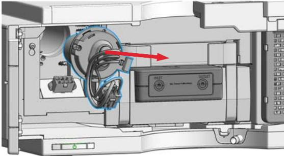
**6** Insert the lamp (RFID tag on the right side).
