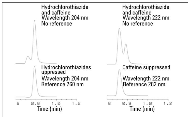
**Figure 25** Peak Suppression Using Reference Wavelength
