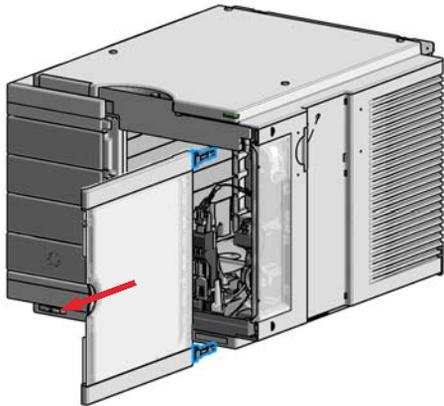
2 For the Installation of the front door. Insert the hinges into their guides and move the door in until the release buttons click into their final position.
