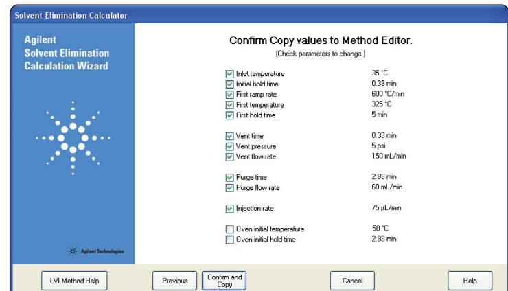
Use the Agilent Solvent Elimination Calculator to develop your solvent vent parameters. Input your solvent choice, injection volume and boiling point of first analyte and suggested starting inlets parameters are calculated for you. Once calculated, you have the choice of copying values to the method editor.
