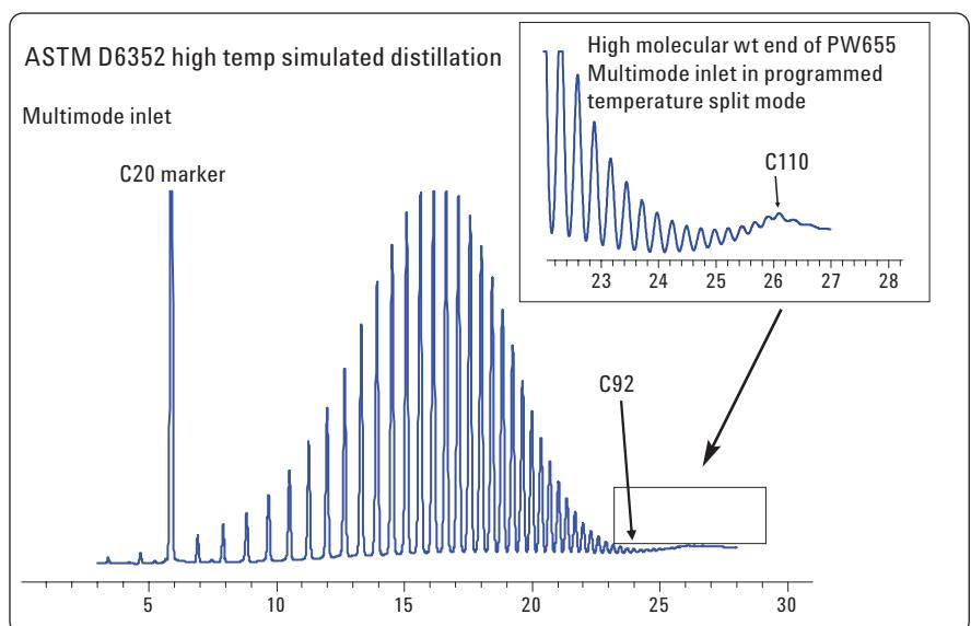
The Multimode Inlet can also be used for High Temperature Applications such as the Automated Preparation of Simulated Distillation Samples for ASTM Methods D2887, D7213, D7398 and D6352 using a Dual Tower 7693A and Tray (Agilent Technologies publication 5990-3778EN).
