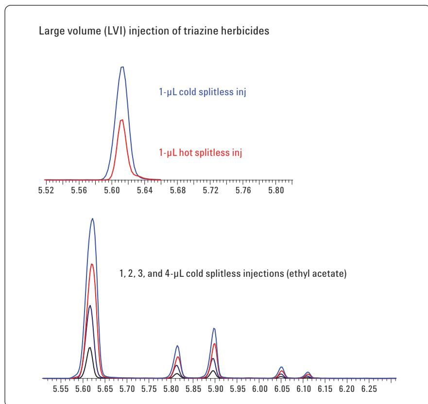
*The top chromatogram using the Multimode Inlet for 1- $\mu\text{L}$  Cold Splitless Injections, response is improved relative to that of the equivalent volume hot injection. In the bottom chromatogram Cold Splitless injection also facilitates larger volume injections while maintaining chromatographic performance.*
