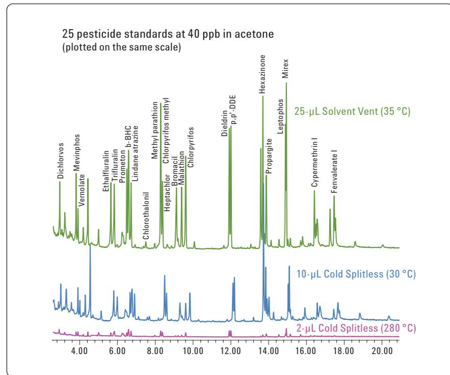
*The power of the Multimode Inlet: Shown on the same scale, total ion chromatograms of test mix indicate the improved response possible using cold splitless or solvent vent mode.*
