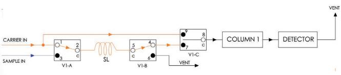
FIGURE 9D: Step 4: Actuating pressure reach 344 kPa (50 psig)
