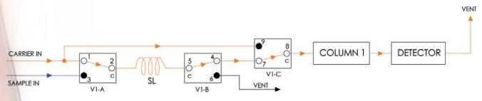
FIGURE 9E: Step 5: Actuating pressure reach 448 kPa (65 psig)
