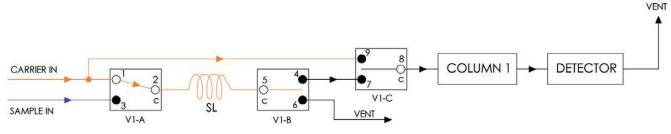
FIGURE 9C: Step 3: Actuating pressure reaching 241 kPa (35 psig)
