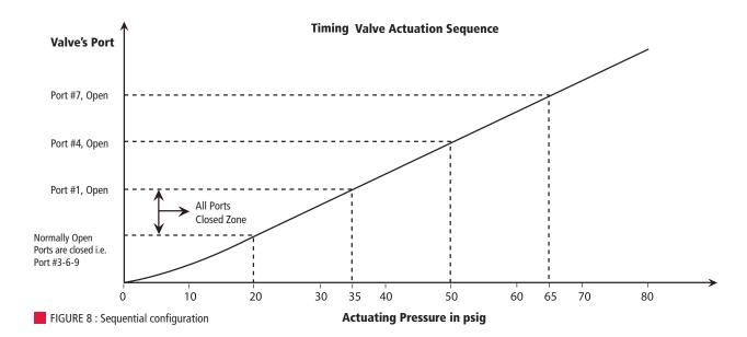
When adjusting the set screws below of the normally closed pistons, sets a compressive force or pressure on the Belleville washer stacks, see Figure 12. Depending on how much pressure is applied on the Belleville washer stacks by the corresponding set screws, different pneumatic pressures will be required to open the corresponding ports. This feature allows the following interesting possibilities.
