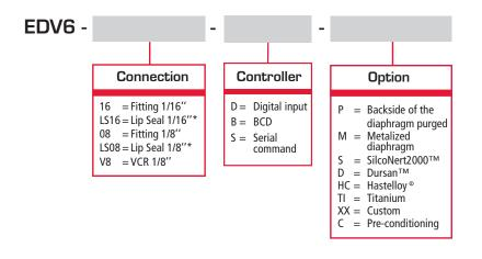
\*Lip Seal: Lip Seal fitting is our new patent pending AFP fitting detail. This reduces the dead volume, eliminates the rotation of the ferrule and improves the sealing resulting in an improved connection for valve and fitting. This is very beneficial for any analytical high sensitivity instrumentation. Sealing integrity of a VCR fitting with the flexibility of a compression fitting. Please refer to Design Report 3 (DR-3) in the Analytical Flow Product Cookbook.
