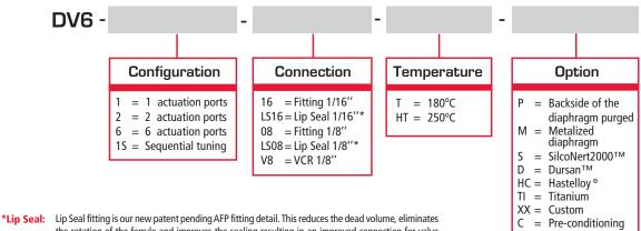
(p) Seal: Lip Seal Intung is our new patent pending APP fitting detail. Inis reduces the dead volume, eliminates the rotation of the ferrule and improves the sealing resulting in an improved connection for valve and fitting. This is very beneficial for any analytical high sensitivity instrumentation. Sealing integrity of a VCR fitting with the flexibility of a compression fitting. Please refer to Design Report 3 (DR-3) in the Analytical Flow Product Cookbook.
