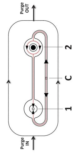
✓ No dead volume effect, continuous sweeping action Purging/Sealing groove design, eliminates
