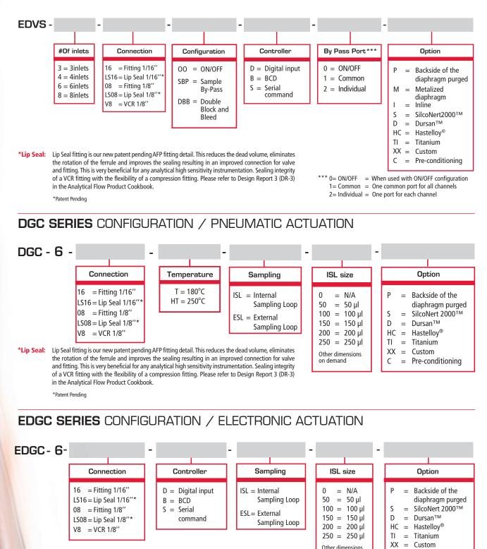
\*Lip Seal: Lip Seal fitting is our new patent pending AFP fitting detail. This reduces the dead volume, eliminates the rotation of the ferrule and improves the sealing resulting in an improved connection for valve and fitting. This is very beneficial for any analytical high sensitivity instrumentation. Sealing integrity of a VCR fitting with the flexibility of a compression fitting. Please refer to Design Report 3 (DR-3) in the Analytical Flow Product Cookbook.
